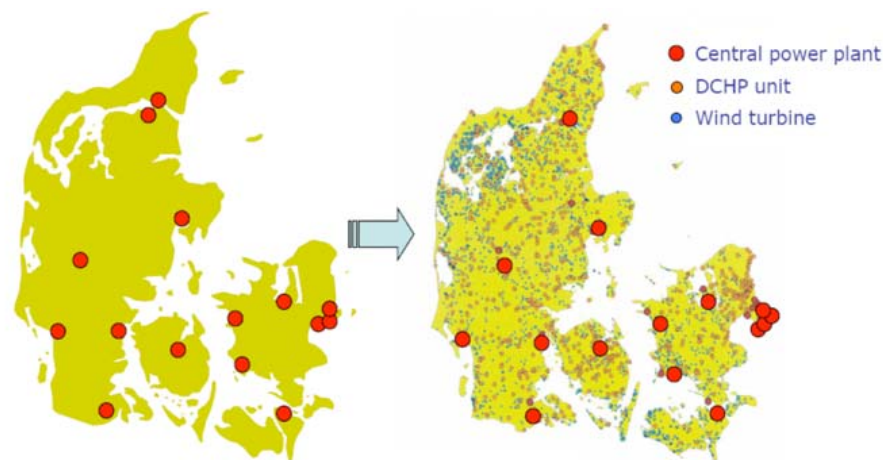
Figure 17: In the 1980s, Denmark relied almost exclusively on central power plants (left). By the 2000s (right), it had transitioned to a system with extensive distributed power (mostly combined heat and power and wind turbines).
